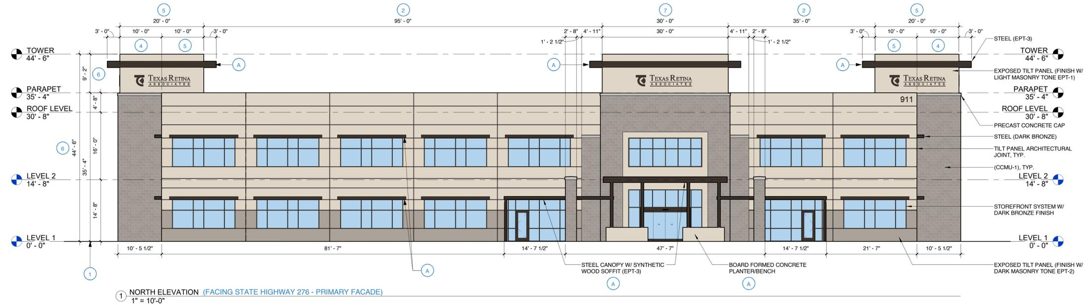
1 NORTH ELEVATION (FACING STATE HIGHWAY 276 - PRIMARY FACADE)
